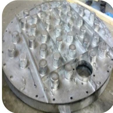
Urea Reactor Super Cup trays
